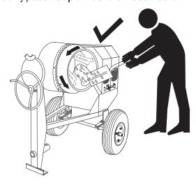
Figure 20. Filling Mixing Drum
